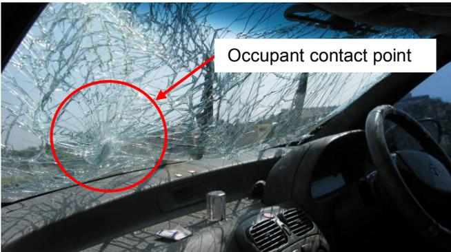
Figure 3B: Roof crush measured is 18 cm and occupant contact identified.
