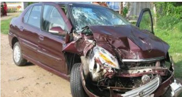
Figure 2: Frontal impact damage
